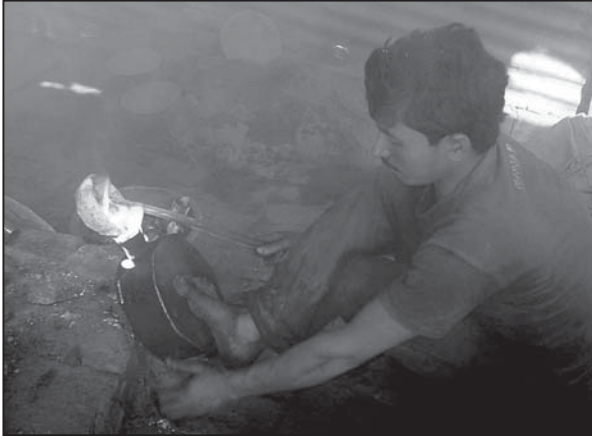
Fig 1: Metal casting work without protection.
